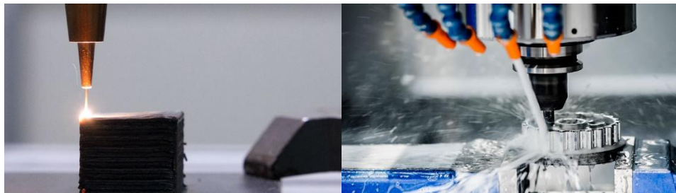
Figure 2: Examples of laser cladding (additive manufacturing) and milling (subtractive manufacturing)
